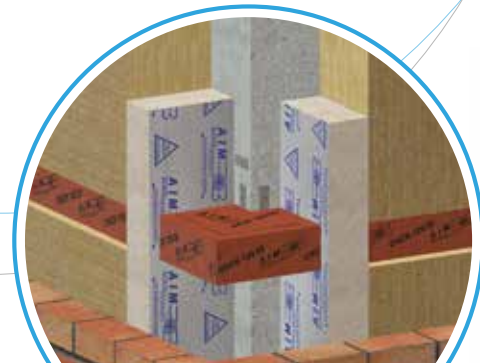
Wall Cavity Fire Barriers forming a vertical corner (Full Fill Cavity)
