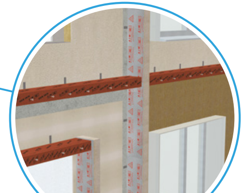
Wall Cavity Barriers and OSCB's working together at a compartment intersection and around a window
