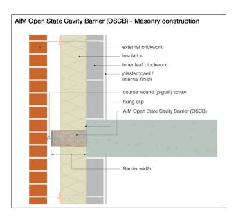
The OSCB 60/25 has also been tested for use vertically in a masonry cavity up to 425mm.
