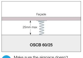
25b Make sure the airspace doesn't exceed 25mm and that all of the coarse wound screws are in contact with the inside of the facade panel
