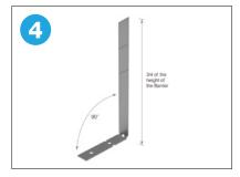
Form two fixing clips to 90° to form an L shape.
