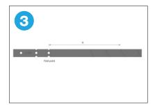
Snap the fixing clips to the correct length. Dimension X should be three quarters of the barrier's height.
