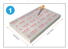
Measure the cavity depth and add 5%. Mark the slab and carefully cut using an insulation saw or hand saw. Please cut in the direction of the arrows printed on the foil facing. Note: This step is not required if installing Wall Cavity Fire Barrier cut to size.
