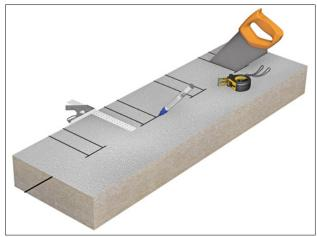
Fit two fixing clips per length of barrier. These should be at roughly 500mm centres. Whilst the barrier really doesn't need fixing clips here, Approved Document B states that all cavity barriers must be mechanically secured in place.
