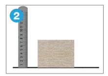
Check that the Wall Cavity Fire Barrier is the correct thickness for the cavity. The barrier should be 5% larger than the cavity.
