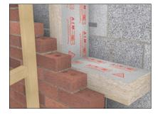
Where vertical barriers could cause "brick push" a push off post or bricklayer profile can be secured to the outside of the building as a preventative measure.
