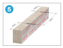
Insert two fixing clips into the barrier at 500mm centres approximately 250mm from each end.
